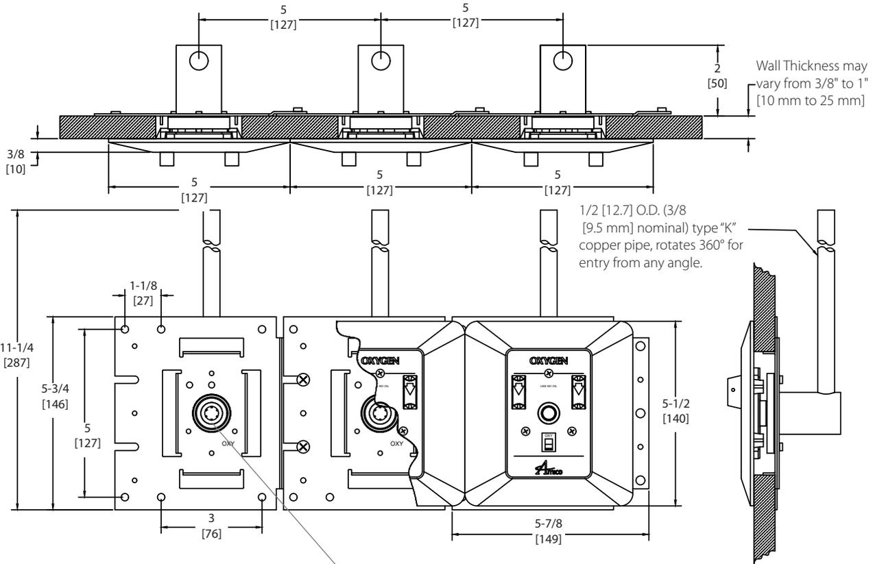
**NOTE:** For CSA/ISO, suction inlets are not supplied with a secondary check valve. A pressure plug is provided for testing purposes, rated at 150 psi (1,034 kPa).
