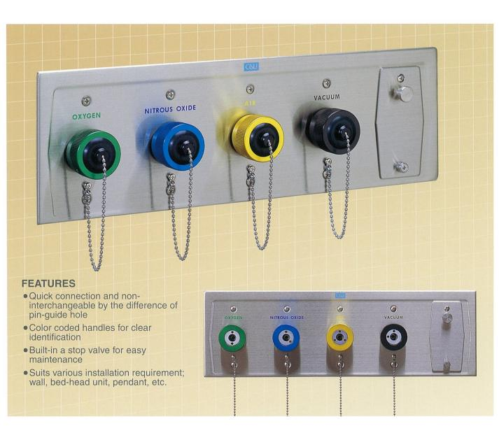
The CPS type wall outlet supplies medical gases more safely and securely at the area, i.e., O.T., ICU, Recovery, ward and so on. An on-wall type to be surface-mounted on the wall, or a in-wall type to be recessed into the wall, is available.
